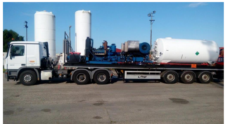
Trailer mounted Nitrogen Unit Hobbs
