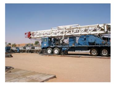
Drilling/Workover rig is designed for: - drilling/workover water wells, oil wells and all relevant operations
